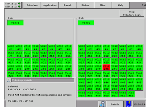
Figure 4 The trouble scan feature gives you a quick overview of the tributaries of the monitored line.
