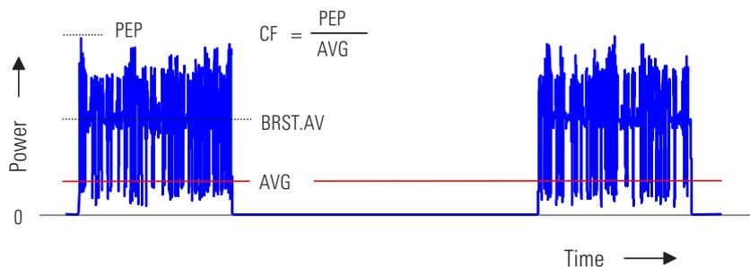
The main parameters of modulated RF shown in the example of a TDMA signal (one active timeslot) with  $\pi/4$  DQPSK modulation:
